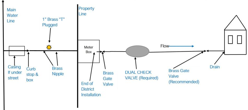
Note: District provides and installs up to and including the meter box. Customer is responsible for all installation after the meter box.
